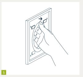
The filter insert is harmonized with Tecanno air vents and can be inserted into recessed and surface-mounted vents (100/125).
